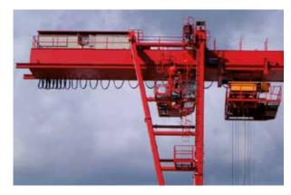
Our festoon systems offer the most flexible solutions for transporting flat or round cables and hoses. A wide variety of profiles and components guarantees reliable installations, adapted to the environment.
