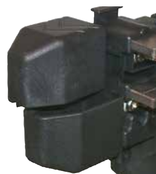
The gliding shoes can quickly and easily be positioned due to the dovetail construction. A visual inspection is possible, for a marking is provided.
