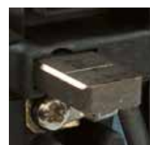
Visual inspection of carbon brushes is rather simple due to the markings as applied.
