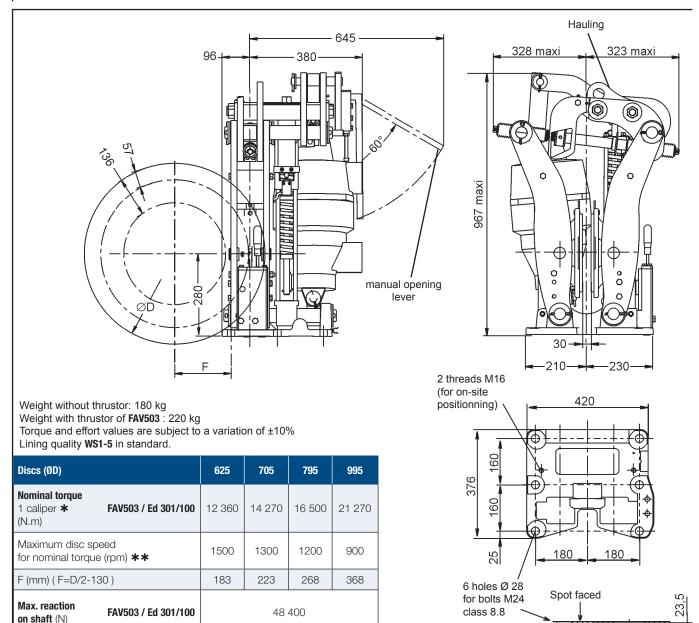
**★** Nominal torque is adjustable from 100% to 70%
